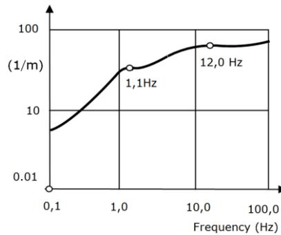
Fig.5 Car frequency response function.
