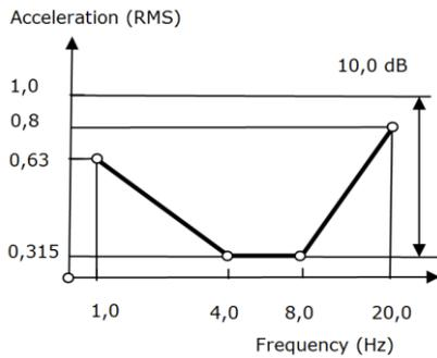
Fig.4 Vertical vibration exposure curve.
