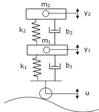
Fig. 3. The two mass passive suspension.
