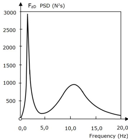
Fig. 2. PSD of the normalized tire load.
