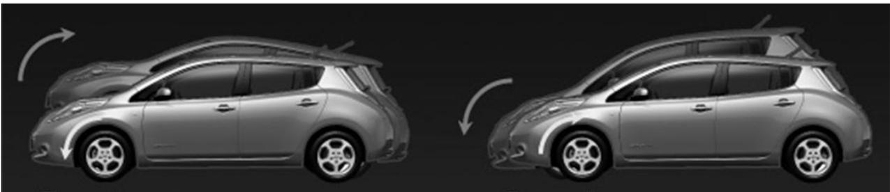
Fig.10 a) torque increase causes raising up the front of the vehicle, b) by torque decrease the front of the vehicle will be lower
